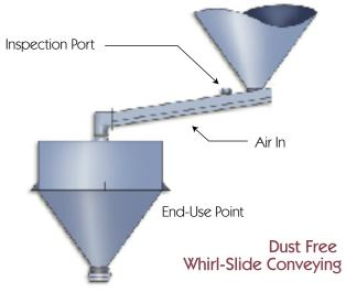
Most powdered products are easily conveyed in the enclosed, dust-free Whirl-Slide. Materials handled by the Whirl-Slide are in the 40 mesh and finer range. Whirl-Slides can be utilized to convey materials from silos or hoppers or other feed points to use points or load out operations like filling rail cars. Whirl-Slides can be used to aerate silos to eliminate bridging.
