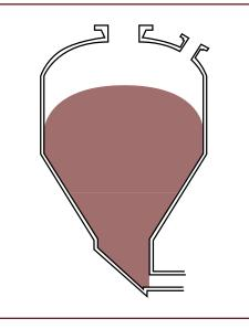
**Blending** - products are homogeneously blended in cycles from two to five minutes using plant compressed air.
