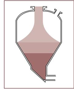
**Filling** - blender is filled by gravity from the batch/scale hopper above. Manual additions can be made using a Whirl-Air manual bag emptier.
