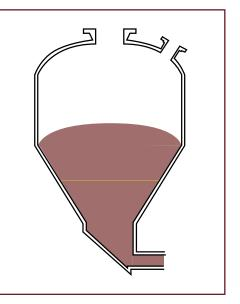
**Conveying** - blended product is pneumatically conveyed to process area. Gravity discharge models are also available.
